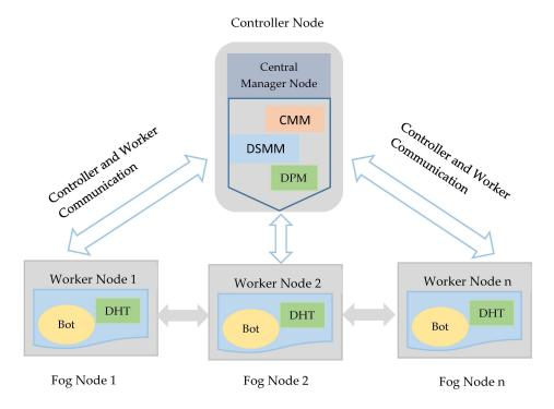
Figure 9. Placement of CMM and DSMM in a controller node.
