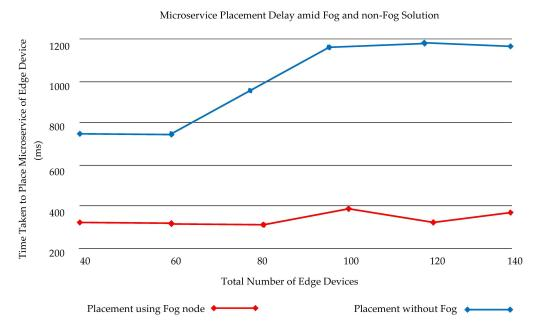
Figure 16. Microservice placement delay in the fog and cloud environment.
