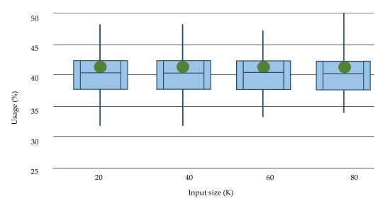
CPU Utilization of Autonomous Bots in Docker Container
