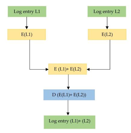
Figure 13. Paillier Homomorphic Encryption (PHE) mechanism in cloud CLS.
