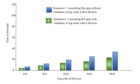
Figure 17. Time taken to place microservice in fog node with four devices.
