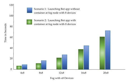
Figure 18. Time taken to place microservice in fog node with eight devices.
