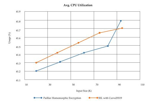
Figure 22. Average CPU utilization for secure log storage using PHE.
